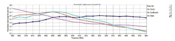
\*\* The indicated read range values are measured in our laboratory testing environment, where antennas with optimum directivity are used with maximum allowed operating power. Different surface materials and environments may exhibit different results.
